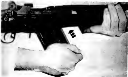
1 Figure 29 Loading the magazine into the rifle.
